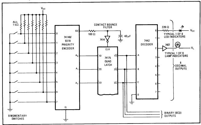
**Interlock.** Momentary switches are interlocked from simultaneous operation by encoding them into a set of latches and then decoding the latch states to drive indicators or other apparatus. Circuit is more reliable than mechanical interlock, and switches can even be remote.
